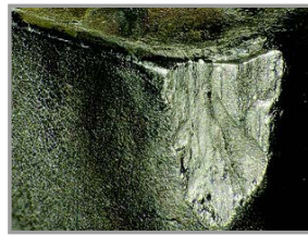
Fracture from welding chipping
